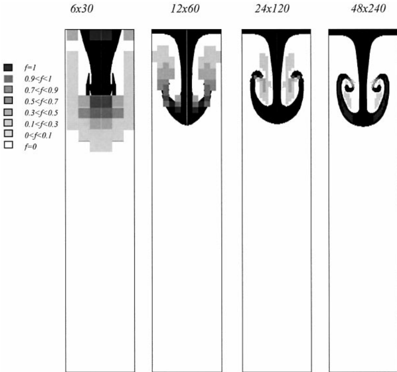
FIG. 26. Grid dependence of the coupled model showed on the state at t = 2.0 .
