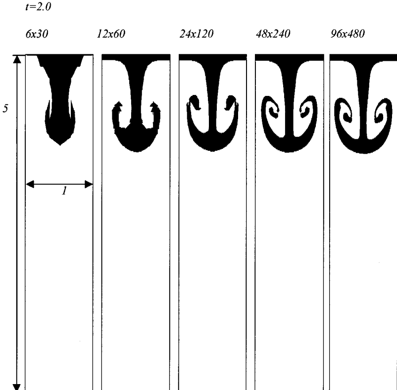
FIG. 23. State of the Rayleigh–Taylor instability at time t = 2.0 simulated with the pure VOF method.
